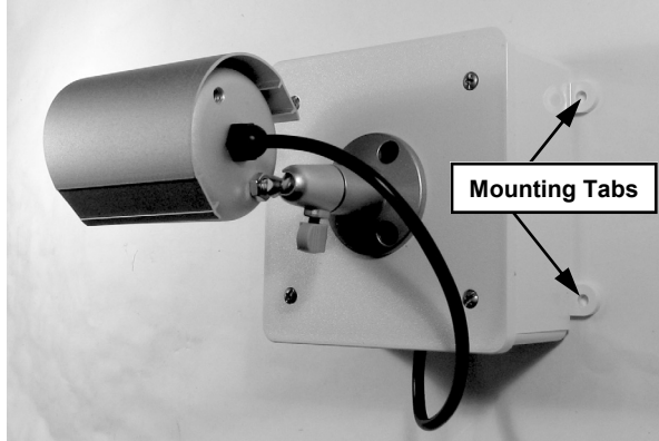
Fig. 8: Create loop when wall mounting
